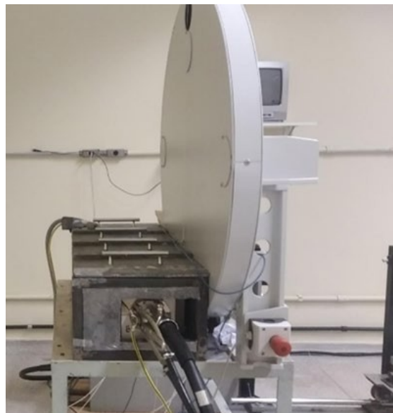
Figure 1: Pantak X-ray irradiator system and PTW filter wheel at LCI/IPEN.
