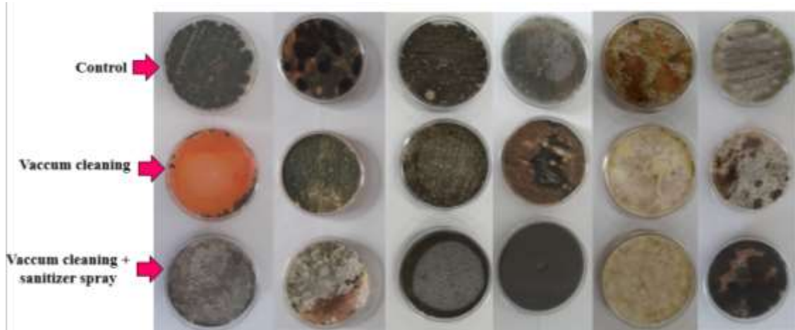
Figure 3: Petri dishes with fungi in control samples, vacuum cleaning and vacuum cleaning and sanitizer spray treatment.
