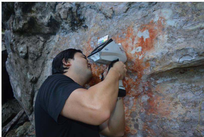
Figure 3. Portable EDXRF Tracer 5i system positioned for measurement on a rock painting.
