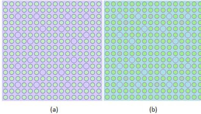
Figure 1: Traditional fuel assemblies (a) UO<sub>2</sub> - (b) UN.
