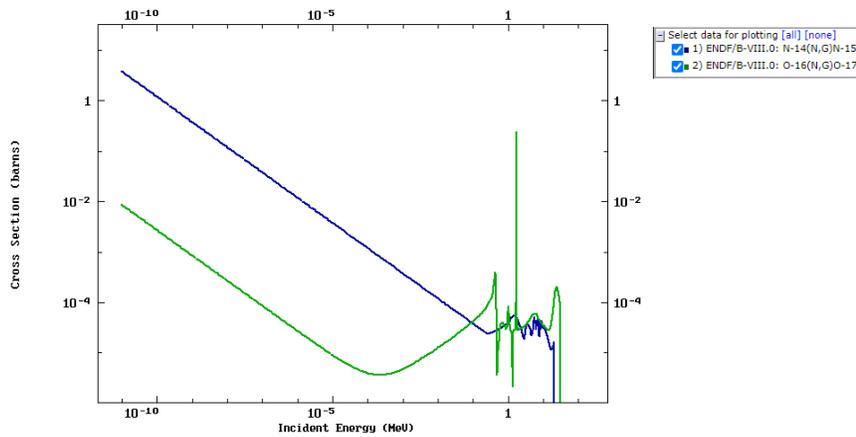
Figure 2: Relation between cross sections (radiative captures) of <sup>14</sup>N and <sup>16</sup>O.
