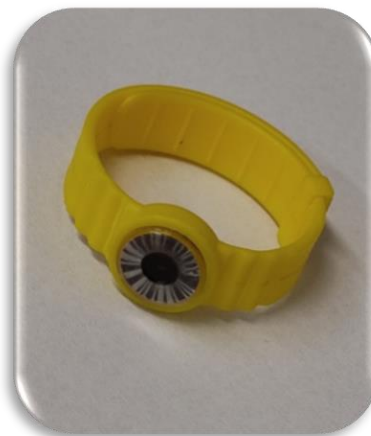
Figure 1: PTFE-Teflon® holder and thermoluminescent detector of LiF:Mg, Ti.
