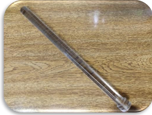
Figure 2: Rod-type phantom used to irradiations in H_p(0.07) .
