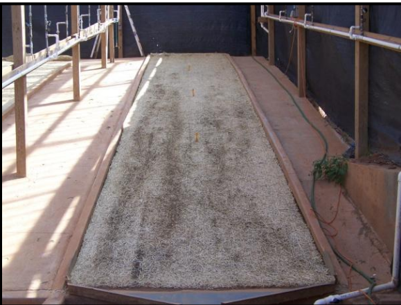
(b) Testing of a geomat (GMA) or rolled erosion control product (RECP)
