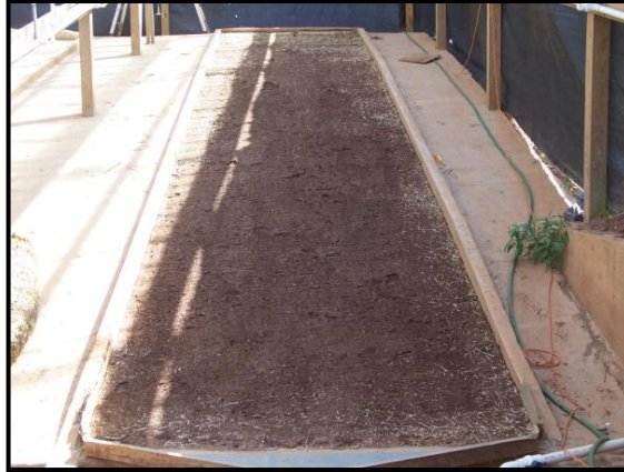
(c) Eroded surface after ECP removed - post test
