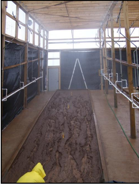
(a) ASTM D6459 Slope Testing facility (bare soils test shown)
