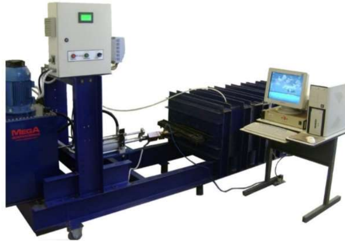
Figure 2. Pullout test equipment (Campos 2013)
