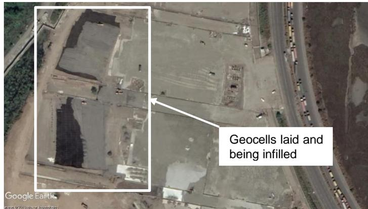
e) Aerial view (Google Earth) of construction of final stage of geocells laid
