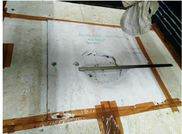
b) Measurement of the indentation on the EPS block
