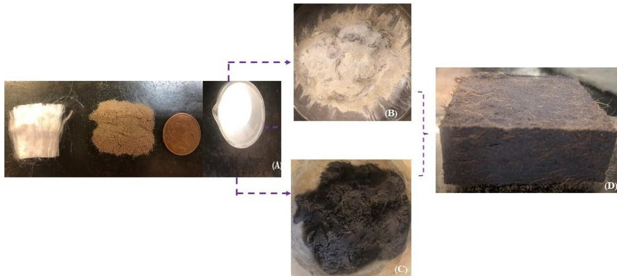
Figure 2. (A) Materials used iron mine tailings, fiber and polymer; (B) iron mine tailings and fiber shredded; (C) iron mine tailings, fiber and polymer mixed; (D) molded specimen.
