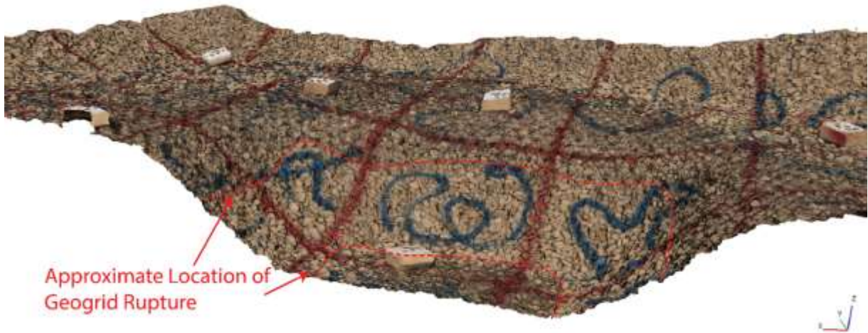
Figure 9: Cross section of photogrammetry reproduced geogrid surface and rupture location
