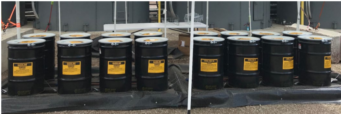
Figure 2. Experimental setup for submersion of geomembrane pouches in fuel drums.
