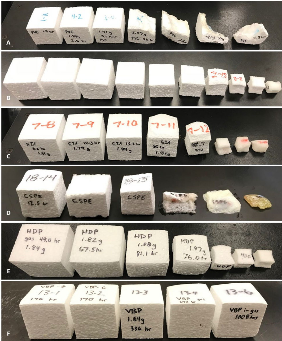
Figure 4. Time resolved geofoam degradation due to gasoline permeation through A) PVD, B) LLDPE, C) EIA, D) CSPE-R, E) HDPE, and F) LLDPE-B geomembranes
