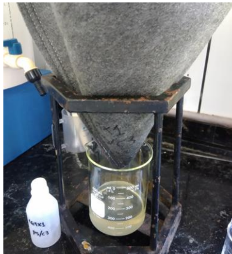
Figure 7. Cone in process of dewatering with polymer.
