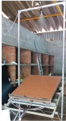
Figure 2 - Overview of the rain simulator equipment.
