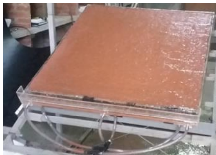
Figure 3 – Surface flow on the unprotected slope
