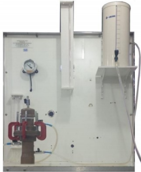
Figure 1. Equipment used to determination of the water permeability characteristics normal to the plane.
