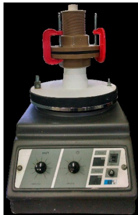
Figure 2. Equipment used to determination apparent opening size.
