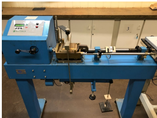
Figure 2. Equipment used in direct shear tests.
