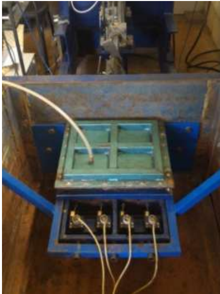
Figure 1. Small box and instrumentation.
