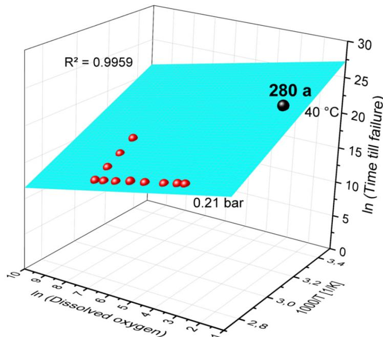
Figure 1. Example of a 3D-extrapolation of a HPAT in an Arrhenius-typical application of the inverse temperature (1/T) over the logarithmic time (ln t) and over the amount of oxygen dissolved in the aqueous medium (ln c(O<sub>2</sub>)).
